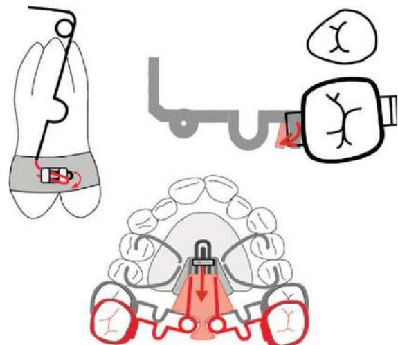
Schematic representation of the Pendulum K with distal screw, integrated uprighting activation, toe-in bend, and distal activation in the Pendulum spring region for bilateral molar distalization.
